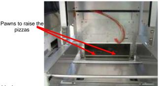
Picture 34 : Oven view (cleaning elements unmounted)
